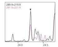
Example of PCBs Analysis in River Water Column: SH-PCB (60 m, 0.25 mm, and 0.25 mm) 2,2', 5,5'-Tetrachlorobiphenyl (#52) (0.080 ng/L concentration in water)
