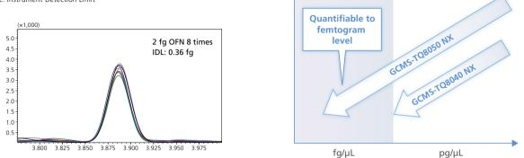
The superior data stability with the GCMS-TQ8050 NX provides sensitivity that rivals high-resolution GC-MS analysis. This powerful new analytical instrument reliably identifies peaks even for trace quantities of dioxins and other substances previously considered difficult to analyze using a quadrupole GC-MS system.
