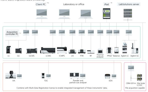
\*1 The acquisition control PC controls analytical instruments. It can also be used to send analytical instructions and perform postrun analysis, just like a client PC. \*2 If a terminal service is used, then LabSolutions software does not need to be installed on client PCs.
